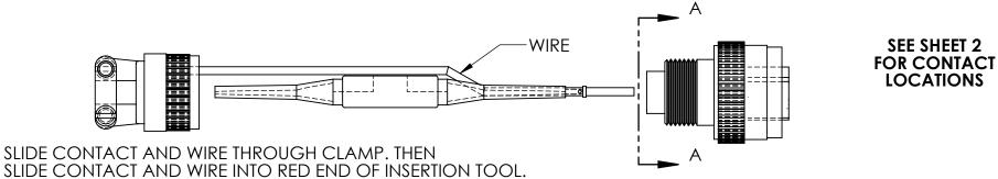
BEGINNING FROM THE CENTER CAVITY AND WORKING OUTWARDS IN A CIRCULAR PATTERN, INSERT WIRED CONTACTS INTO PLUG. (SEE FIG 4 (VIEW A-A) ON SHEET 2 FOR CONTACT LOCATIONS.) PUSH TOOL STRAIGHT INTO CAVITY UNTIL CONTACT SNAPS INTO POSITION. A LIGHT PULL ON THE WIRE WILL ASSURE THAT THE CONTACT IS SECURELY IN POSITION. REMOVE INSERTION TOOL AND REPEAT.
